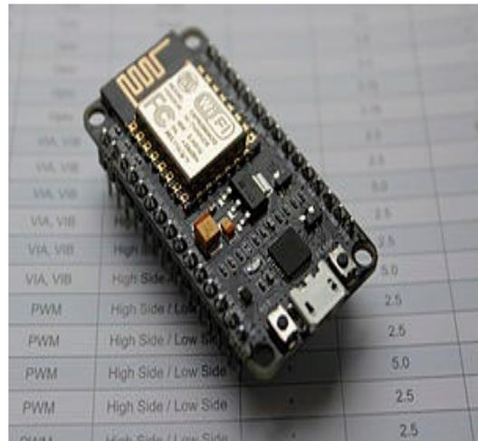
Figure 9: Node MCU Esp-8266
