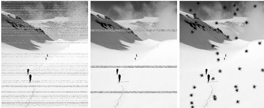
Figure 10.4. A variety of other natural spatial noise models. We show two versions. The first image shows the result of randomly replacing lines with noise, where the probability of replacing the line is uniform; in the second, a block of lines of random length is replaced with noise — this process is a reasonable model of the sort of noise that occurs in fast-forwarding or rewinding VCR’s. In the third, a Poisson process chooses “noise points”; in a neighbourhood of each noise point, pixels are randomly marked black with a probability that falls off as the negative exponential of the distance from the noise point. This process simulates damage to the CCD array, or to the lens.
